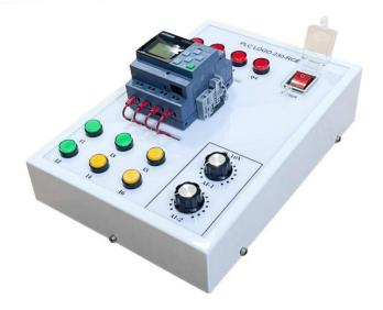
The PLC LOGO 230-COM with CMK 2000 trainer is the compact trainer devices that provide users with an introduction to logical signal processing within a mini control system.
