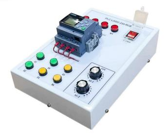
The PLC LOGO 230-COM1 with CSM 12/24 trainer is the compact trainer devices that provide users with an introduction to logical signal processing within a mini control system.
